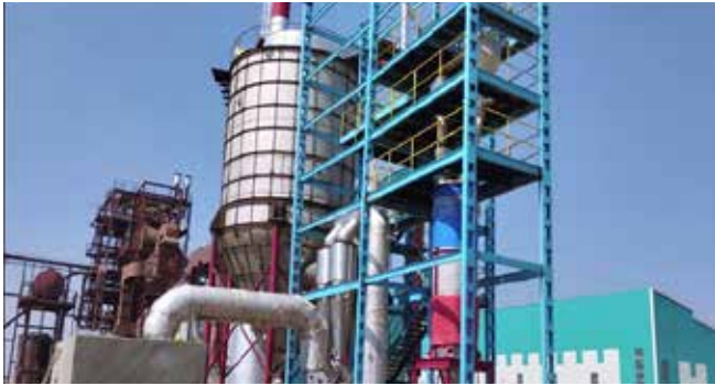
Spent Wash Dryer: The spent wash generated from the distillery is fired in the dryer and converted into powder, which contains high volumes of potash - a key source of fertilizer. Due to this we have achieved ZLD, i.e. Zero Liquid Discharge, in the distillery.
